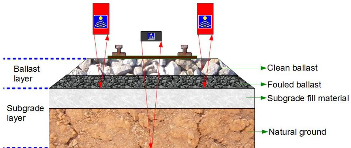
Simplified railroad cross section with GPR antennas positioned over the areas of interest
